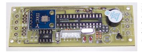
Note the « + » sign on the buzzer do not reverse it (remove the tape and check that you also have a + sign on the plastic cap). The "+" sign should be also the longest leg.
