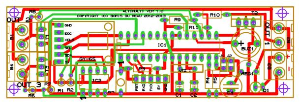
An epoxy board is provided with the kit, all components are drawn so that they can be quickly identified. This is a single sided board. This means that you only need to solder the components on one side.
