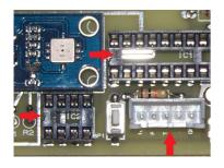
If the socket has been correctly soldered use the socket mark to place the microcontroller and align both marks.
