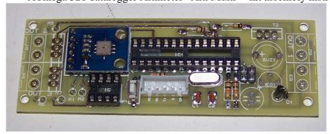
Without a diode if you reverse the voltage by mistake (ie: when you plug the battery) then the circuit will be permanently damaged.
