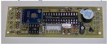
The 2 small one are the 22pF and they are around the crystal. However the  $47\mu F$  capacitor has a \* + \* which should go up, the other leg being connected to the ground at the bottom.
