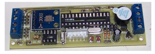
Make sure that the terminal blocs output are facing each end of the circuit board.
