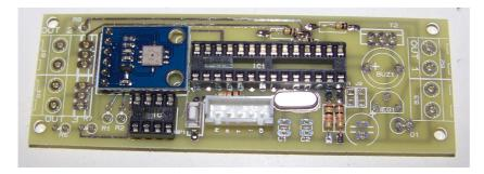
If it has not been done already; cut the connectors so that one is 6 pins and the other two are 2 pins. Then plug them to the board. Use cella tape to hold them while you are soldering. Make sure the connector is soldered like in the picture.
