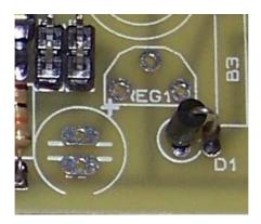
The protection diode has to be correctly plugged. The silver ring should be at the bottom, touching the board.
