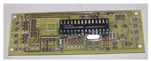
Plug the 28 pins socket and make sure that you do not miss any pin. You have a mark on the socket make sure it is on the left, this will help you later on when you plug the micro controller. Check the photo to position it.
