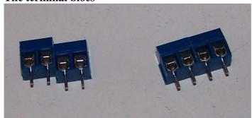
The terminal bloc can be clipped together.
