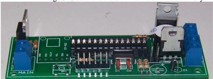
The 2 small one are the 22pF and they are around the crystal. However the  $47\mu F$  capacitor has a « + » which should go up, the other leg being connected to the ground at the bottom.
