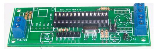
Make sure that the terminal blocs output are facing each end of the circuit board.
