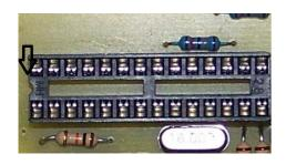
If the socket has been correctly soldered use the socket mark to place the microcontroller and align both marks.
