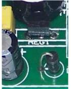
The regulator flat face should be facing the diode and capacitor.
