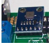
You need to solder that board directly on the altimeter board.
