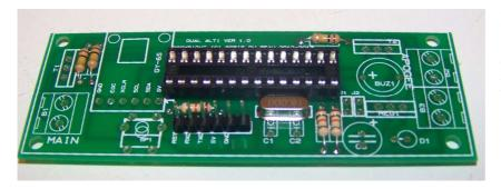
If it has not been done already; cut the connectors so that one is 6 pins and the other two are 2 pins. Then plug them to the board. Use cella tape to hold them while you are soldering.
